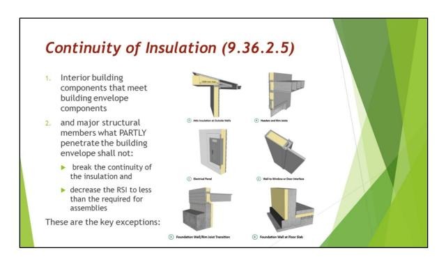
Interior building components that meet building envelope components and major structural members what PARTLY penetrate the building envelope shall not:
